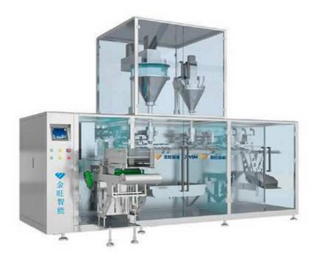
DGD-280AJ automatic horizontal bag feeding bagging machine is an online weighing bagging machine newly developed by our company. Under the programmable control of PLC, the functions of bag taking  $\rightarrow$  bag opening  $\rightarrow$  detection  $\rightarrow$  filling 1  $\rightarrow$  filling 2 (weighing)  $\rightarrow$  sealing  $\rightarrow$  finished product are realized.
