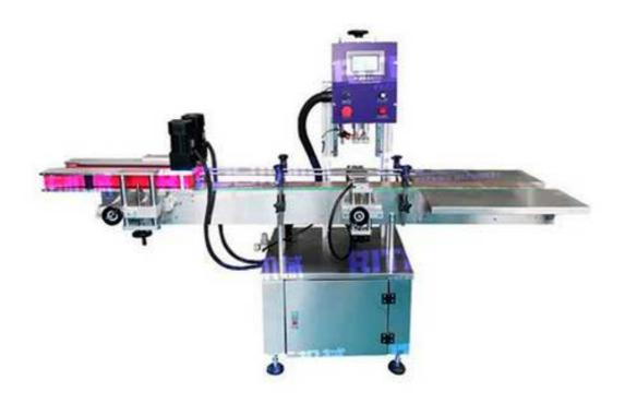
Bottle capping machine adopts double motor design, easy operation, simple maintenance, reliable operation, large applicability, its working principle is to clamp the bottle body through the cylinder, and the double motor drives four groups of friction wheels to rotate the bottle cap to achieve the purpose of tightening the bottle cap.
