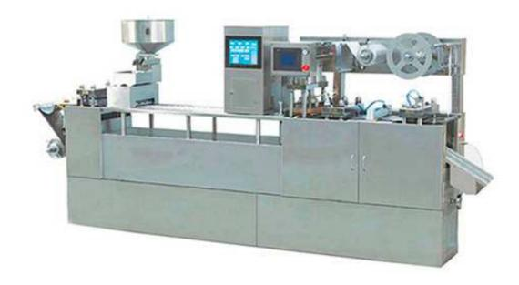
This machine adopts PLC control, man-machine interface operation, frequency conversion speed regulation, high degree of automation and easy operation.
