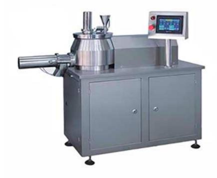
HLSG-400 High shear mixer granulator is a new generation of granulating equipment developed by our company, which can finish the procedures of mixing, wetting, granulating in one time. Which is very effective and in compliance with GMP standard.
