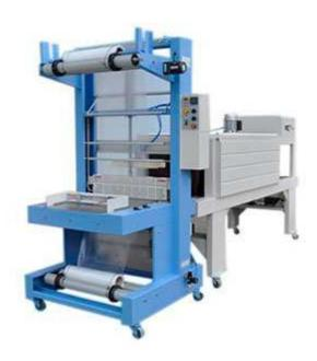
TF6540SA+BS5540M Sealing & Shrinking Packaging Machine is semi-automatic sealing packing machine. The semi-automatic sealing and shrinking packaging machines is suitable for PE film packing. Compared to the traditional carton packaging, it has significant savings in packaging costs.
