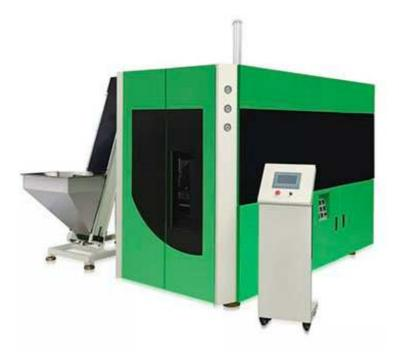
This Linear PET Bottle Blowing Machine Mainly Be Used For Water And Beverage PET Bottle Blowing. Speed From 500bph-6000bph For Various Bottle Shape And Bottle Volume From 100ml-25L.
