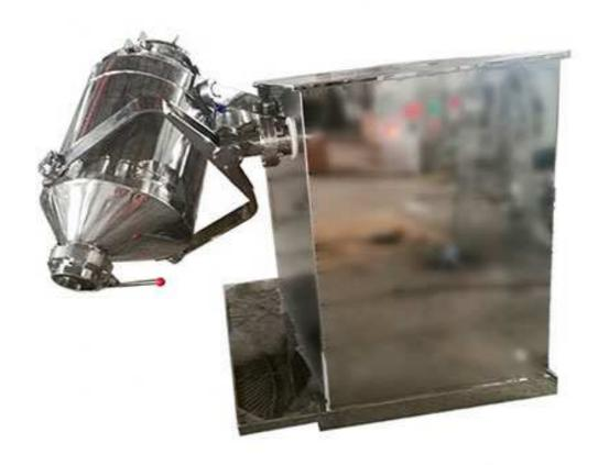
3D swing Mixer Machine is suitable for mixing dry powder materials with high mixing uniformity and good mixing effect. The barrel is driven by the shaft to move and roll so that the material in the barrel moves in three directions to achieve the effect of mixing. The Stand Mixer can be used to mix food powder, it is the dry powder Food mixer with the best mixing effect.
