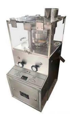
This machine is a kind of single pressure automatic rotating continuous tablet pressing machine, it will press granular raw materials into various tablets, mainly used in the pharmaceutical industry of tablet production, at the same time for chemical industry, food industry, etc. The outer cover of the machine is fully enclosed and made of stainless steel. The surface of the turntable is specially treated to keep the surface gloss and prevent cross contamination.
