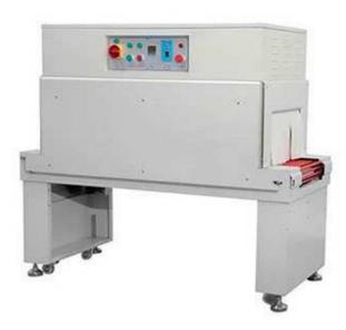
The heat shrinkable tunnel and heat shrinkable packaging machine are used together. After the packaging materials are packaged by the heat shrinkable packaging machine, they are heated in the heat shrinkable tunnel. Under the action of high temperature, the heat shrinkable film produces obvious shrinkage phenomenon, which makes the original relaxed packaging tight and forms a very beautiful packaging effect.
