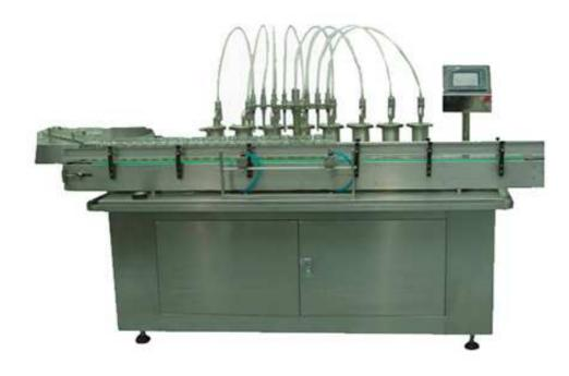
This machine is the main filling equipment of liquid filling production line, which is mainly applied in the filling of 50 - 500 ml glass bottle or plastic bottle.
