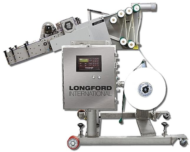
These high speed feeders are specifically designed to feed coupons, backer cards etc., from a roll format and cut them to the proper size and feed them into the packaging stream. The coupons can be fed flat or folded (half fold, "Z" fold, and "W" fold) and the feeder can create a "U" board from the backer stock. The RF375 has unmatched labour savings and can operate up to 8 hours without loading another roll. Also available in stainless steel washdown configuration.
