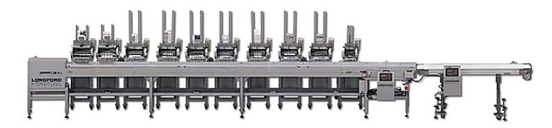
Design/build a modular, flexible system that is able to collate, fulfill and (optionally) overwrap printed media, software collateral ready for distribution. Use friction feeders capable of being moved from line to line, plant to plant in a collating format. All feeders can 'plug and play' on this line or on any other conveyer. Line controller insures feeders dispense on time and in sequence.
