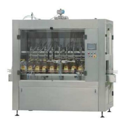
This Type filling machine is a high-tech product designed and developed by our company. It suits for different viscosity of water agent, semi-fluid and paste, it is widely used in the product filling of foodstuff, cosmetics, medicine, grease, daily chemical industry, detergent, pesticide and chemical industry. Using the straight filling way, may be used in the different vessels, needn't add any parts.
