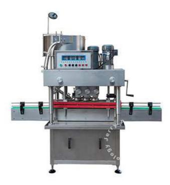
This In-line Structure Capping Machine is making up with cap sorter, cap falling rail, bottle-tightening structure and capping wheels. By the tightening of the belts, the bottles finish the movement of cap scratch, push and capping. It applies to the capping of round and flat bottles. This capping machine is with easy structure and adjustment. When changing the bottle type, you do not need to change the spare part, only adjustment is enough.
