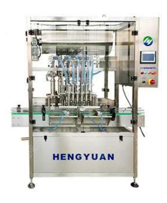
Automatic Linear piston granuled sauce filling machine is for different viscous liquid and cream with different bottle or jars. The performance of the product reaches the international leading level. PLC control, servo motor driving, equipped with brand touch screen, smooth operation, no leakage phenomenon, No bottle no filling, automatically control feeding the liquid into machine tank, liquid level is controlled at the same height.
