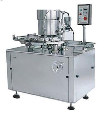
KGL-1 is the first generation of roller capping machine which our company has developed by referring the similar product in domestic market. After several innovations, it is deeply welcomed by pharmaceutical factory users. It is suitable for the capping of round glass bottle and plastic bottle. It is used in pharmaceutical industry, light industry and chemical industry.
