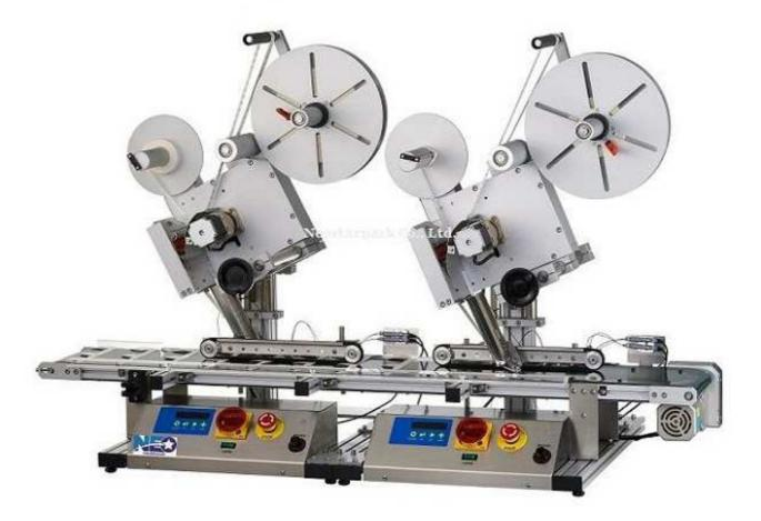
Tabletop Top And Side Labeler NLT-1252 with two label applicators on one conveyor. Tabletop Top And Side Labeler is suitable for various flat products such as plastic boxes, DDR, cassette's, food products note book, aluminum foil bags, etc. It can be connected with production line to elevate production.
