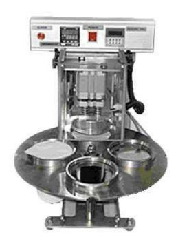
Performance: Manual sealing machine for Pre Cut Aluminum lids
