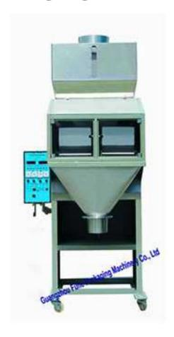
It is used in corn, wheat, urea, ore sand, compound fertilizer, etc grain product ration packing machine.
