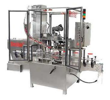
The NRS-51-HES is a heavy duty, self-contained, versatile, automatic "chuck" style capping machine - designed to apply large size caps (70-120mm) with easy change over. The NRS-51 capping machine runs at speeds up to 60 per minute; limited only by container, cap, and product.
