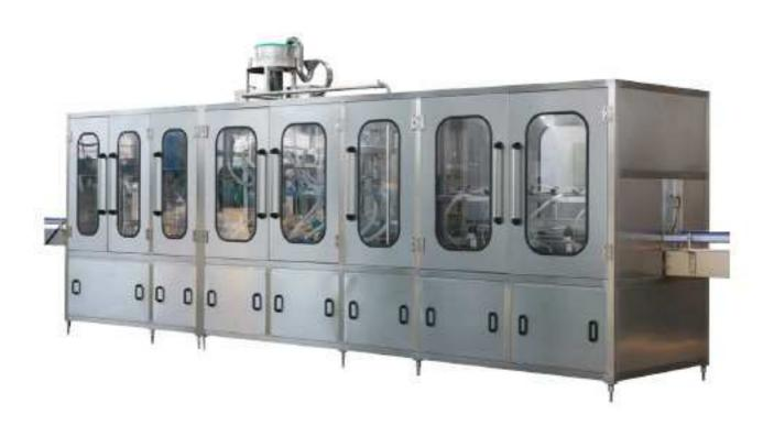
This Machine specially for 3L - 10L Big bottle drinking water, It integrates bottle washing, filling and capping into one unit. All parts of this machine is made of high quality stainless steel materials, it cannot cause rust to influence the filling beverage, it not only reach the standard of sanitation, but also prolong its using life.
