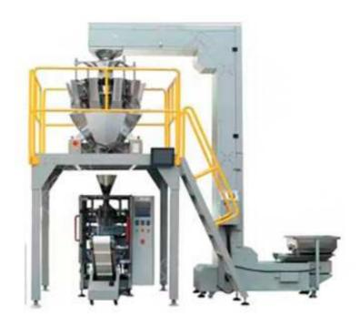
This automatic chips packaging system, integrating 10 head combination weighers, infeed&takeaway conveyors, is suited for chips packing, nut packing, snacks packaging.
