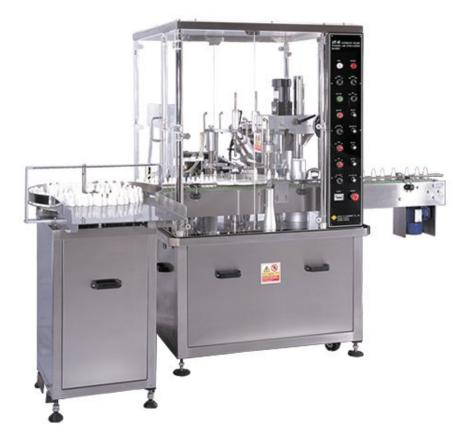
The liquid packaging equipment compliances with cGMP liquid production guidelines and the common application is for below 60mL low viscosity products.
