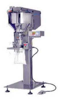
Independent drive through motor controlled by electronical speed inverter, Independent stirring rods, Auger dosing implements provided with "clapet" closure to avoid leakages, Supply funnel level, in order to control the devices of the product supply to the dosing unit, Weighing platform equipped with weight cell, Control box equipped with CPU microprocessor provided with the following applications:
