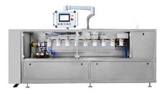
The main packager can be integrated with various filling systems, suitable for all kinds of products, such as powder, small granule, liquid, viscous liquid, block, stick and irregular products.
