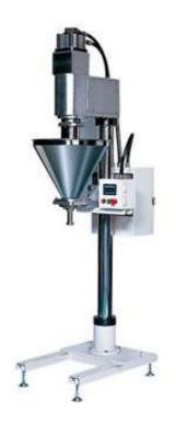
The FRT filling machine is designed explicitly to be used with a short auger for the specific purpose of filling toner and to be used semi-automatic.
