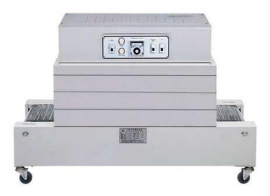
The small shrink tunnel is suitable for shrink films such as PVC, PP, POF, etc. There are shrinking tubes on the top, bottom and sides of the shrinking room. The temperature of the shrink room and the speed of the conveyor are adjustable. And the size of the machine can be customized.
