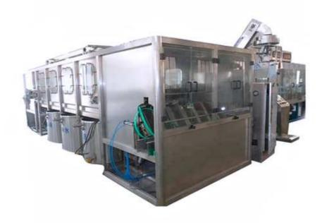
This automatic mineral water filling machine mainly used in the water filling operations, the three function of bottle washing, filling and capping are composed in one body of the machine, the whole process is automatic, it is conveniently trunked to adjust the machine to fill various types of bottles, the filling operation is faster and more stable due to the advanced filling valve technology, The famous brand programed controller (PLC) is adopted to control the machine runs automatically.
