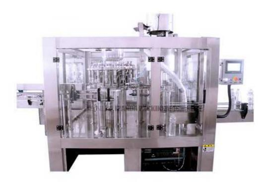
The machine is advanced filling and capping equipment, it's designed on the basis of absorbing domestic and foreign advanced technology. It is mainly used in filling and capping carbonated beverages like soft drinks, cola, sparkling wine, etc. It has such advantages as advanced construction, stable working, convenient operation, and repair & maintenance, transducer control as well as high production efficiency. It is the ideal equipment for mid-scale & small-scale beverage factory.
