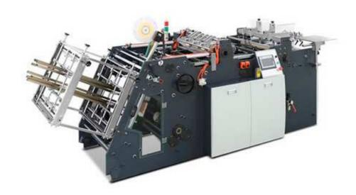
PB-600 automatic paper box erecting forming machine is designed to erect and form paper box like hamburger box, take-out box, food tray, lunch box, French fries box, noodle box, hot dog box, etc. This machine is versatile and can form different types of boxes.
