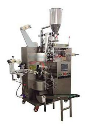
Inner bag is made of filter paper with thread and tag attached, and outer bag is made of composite paper. The biggest advantage is: tag attaching and outer bag making can adopt photoelectric positioning.
