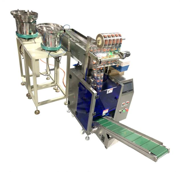
The counting packaging machine is dedicated for counting, filling and packaging of small items, such as nails, nuts, screws, plastic spoons, wall plugs or fixings, washers, small spare parts, small hardware, small electronic components, and all small items in pillow-shaped, 3-side sealed bags. The whole package processes is packed items into the counting bowls with vibrating to feed into the conveying bucket hopper by the track feeding; usually each item needs one counting bowl at least;
