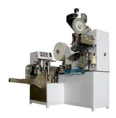
This is our high speed automatic tea bag packing machine, it makes filter tea bag with cotton thread and tag, the speed 110 bags/min. There is auto boxing device, vacuum feeding device, heat sealing tag device, stirrer, date printing machine optional.
