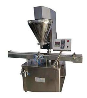
Automatic Auger type Powder filling machine is precision built on sturdy welded MS frame completely enclosed in stainless steel sheet and doors are provided to facilitate the servicing of machine. The unit is made compact, versatile and enclosed in stainless steel elegantly matt finish body.
