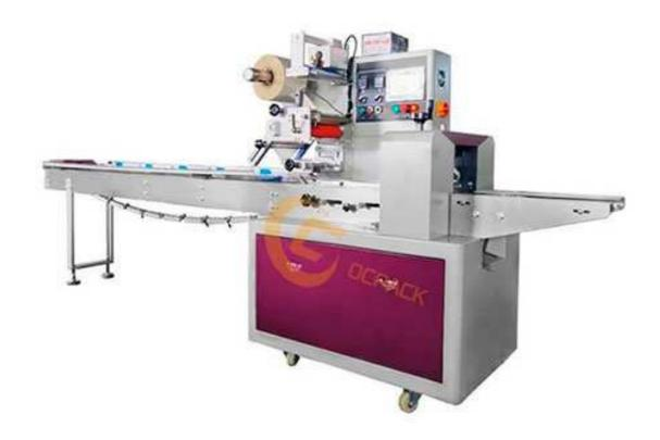
Horizontal up film roll pulling type packing machine for product like bread, biscuit, cookies, chocolate, candy etc. PLC touch screen control, different language customize for customer, according to your product size to choose the suitable model. Back sealing pillow bag, can be add with nitrogen gas filling.
