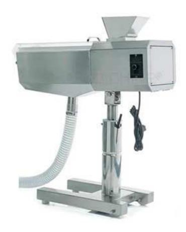
The SWS-137 high-speed tablet sieving machine adopts compressed air for scavenging, centrifugal dust removing and roller edge grinding principle to eliminate dust on the tablet surfaces and edge burrs, so as to make the tablet surfaces clean and the edges neat.
