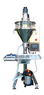
Semi-automatic Free Standing Auger Filling Machine is mainly composed of auger filler head, free standing structure, control cabinet, driving motor, weigher etc. The semi-automatic auger filling machine is usually used for powdery or fine granular products quantitative metering and filling for premade bags, bottles, cans etc.
