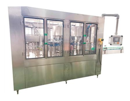
This series of machines are applied to the production of pure water, mineral water, it integrates bottle washing, filling and capping into one body of the machine. It is very convenient to change bottle size by means of advanced bottle conveying technology—bottle neck clamping & bottle suspending technology.
