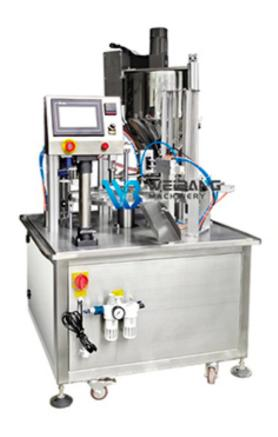
This machine is the mufti-functional and advanced yogurt cup filling machine. It is featured with automatic dispensing cup, filling, sealing, cover pressing. It is suitable to milk, juice, honey, water and granular, powder, fruit, crisp and so on.
