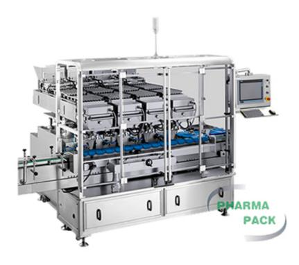
It's an automatic counter. Small footprints allow it to integrate into any packaging line. It's an automatic tablet counter that counts and bottles at the same time to improve production efficiency.
