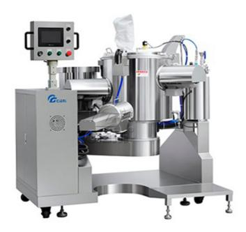
Designed for mixing cosmetic powder, it can mix 10-25kgs at a time. It applies to cosmetic, pharmacy, chemical industry, dyestuff, and plastic industries. The machine mixes the material quickly and equably under effective of homogenizing and stirring.
