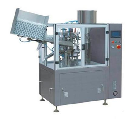
The machine can automatically orientate eye marks, filling, sealing, pressing date and cutting the end.
