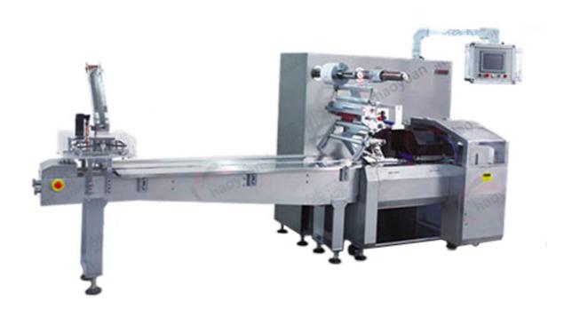
This machine is based on the common reciprocating pillow type packaging machine, which is controlled by full servo motor, improved structure, increased packaging speed, and added multiple detection and elimination, fault self diagnosis, alarm and shutdown, remote control and other functions, greatly improving the production efficiency, reducing personnel and production costs.
