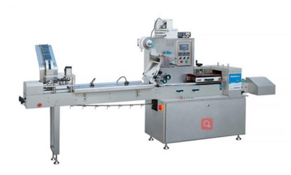
The equipment is simple in appearance and beautiful in shape. The overall external cover is made of 304 stainless steel, which fully meets the requirements of GMP in pharmaceutical industry. Each rotating part is covered by a shell, which will not cause harm to human body. The whole frame adopts many pieces of welding after the whole processing molding, so it is not only simple and generous, and the strength and stiffness has been greatly improved.
