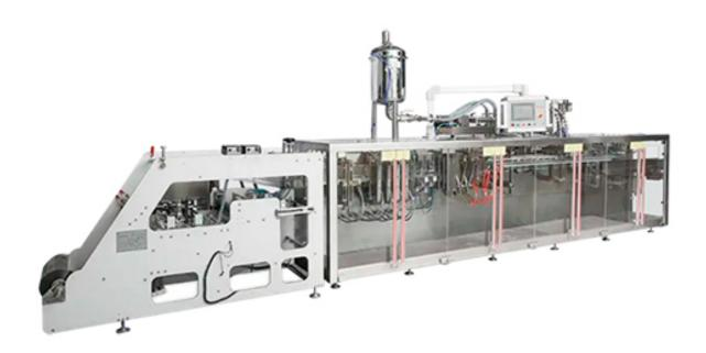
BHD-280DS is specially designed for standard stand-up pouches, and can produce and package two bags at the same time. As the bag size and filling volume increase, the packaging speed also increases, and the packaging accuracy remains unchanged. It is often used for packaging melon seeds, cereals, laundry beads, etc. Wide range of packaging.
