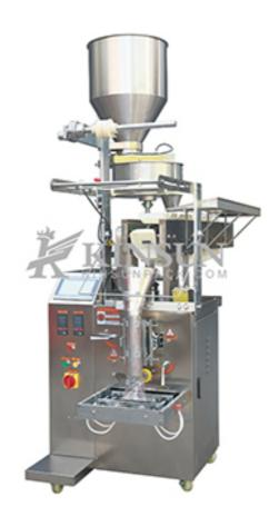
The fully automatic powder packaging machine is suitable for fully automatic packaging of powders or fine particles in products in industries such as medicine, food, daily chemicals, pesticides, and hardware products.
