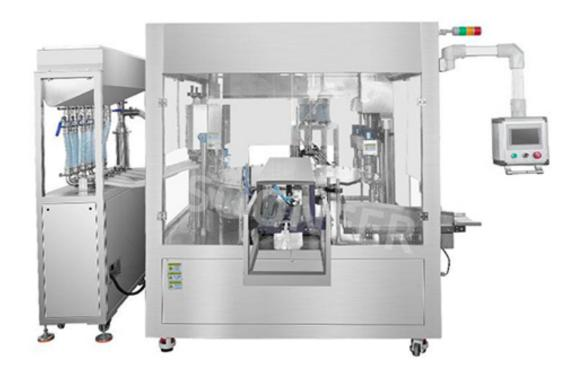
The spout pouch filling and capping machine is a specialized packaging system used to fill and seal liquid or semi-liquid products into spout pouch.
