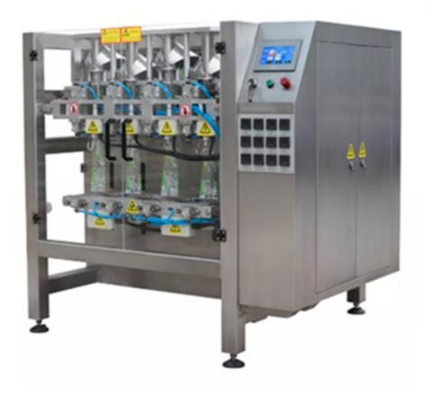
Dustial Machinery® 4 Lanes Vertical Packaging Machine is suitable to use in automatic packing loose solid material, such as snack food, nut, popcorn, seed, sugar and salt etc. which shape is roll, slice and granule.
