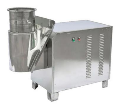
This machine adopts one pair of rotating grinding blade to grind form damp material into columnshape granule by stainless steel sieve cylinder which is provided to pelletize in next process.
