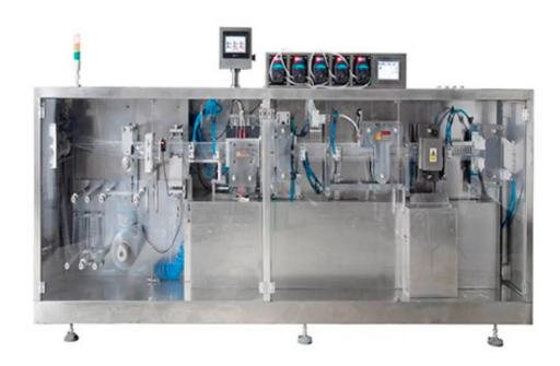
High capacity, high speed, high precision, and advanced motion controller. Stepless frequency conversion speed regulation control. Servo motor controls film traction device.
